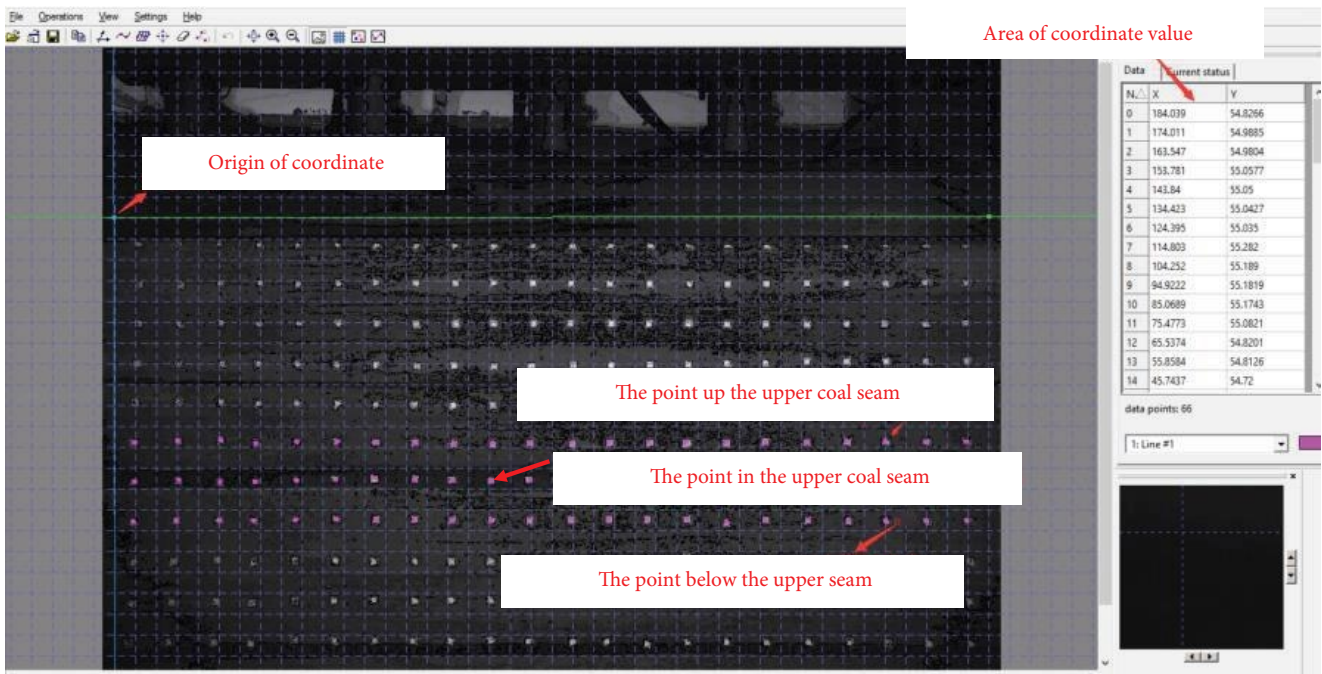
FIGURE 14: The measurement of the relative coordinate of the measuring point.
