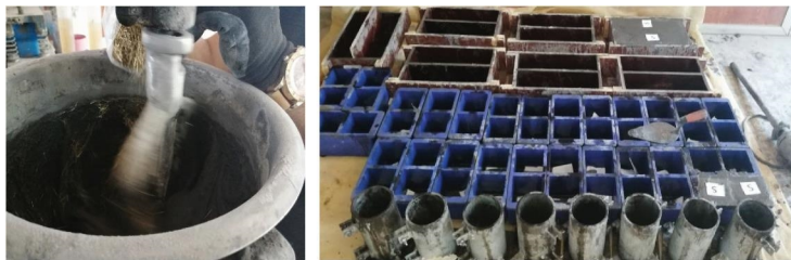
FIGURE 5: Mixing procedure and casting of RPC.
