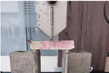
FIGURE 8: Three-point test of the specimen.
