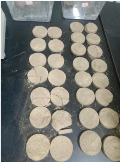
FIGURE 6: Specimen form after shear test.
