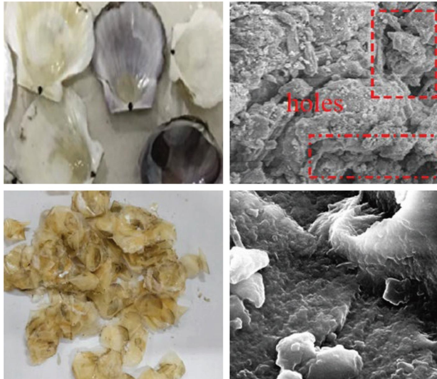
FIGURE 15: Macro- and microstructure of bioshell.
