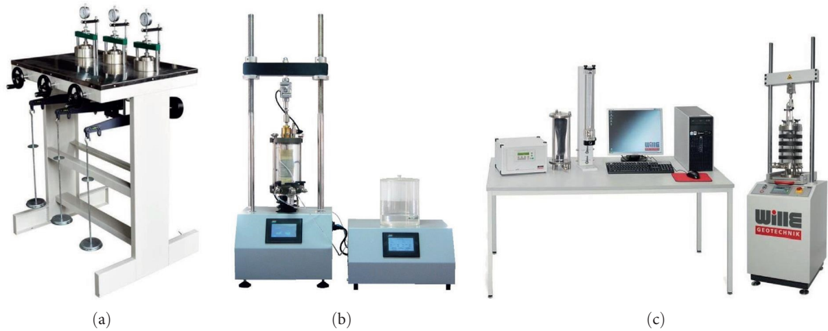
FIGURE 3: (a) Single lever soil consolidation instrument, (b) strain-controlled direct shear instrument, and (c) dynamic triaxial testing instrument.
