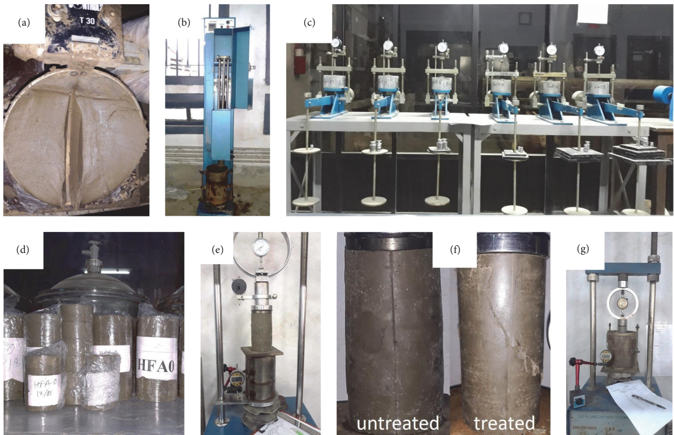
FIGURE 3: Illustration of various experiments: (a) liquid limit test, (b) mechanical compaction device, (c) swelling pressure test assembly, (d) curing of UCS specimens, (e) UCS test device, (f) typical failure of UCS specimens, and (g) CBR test.
