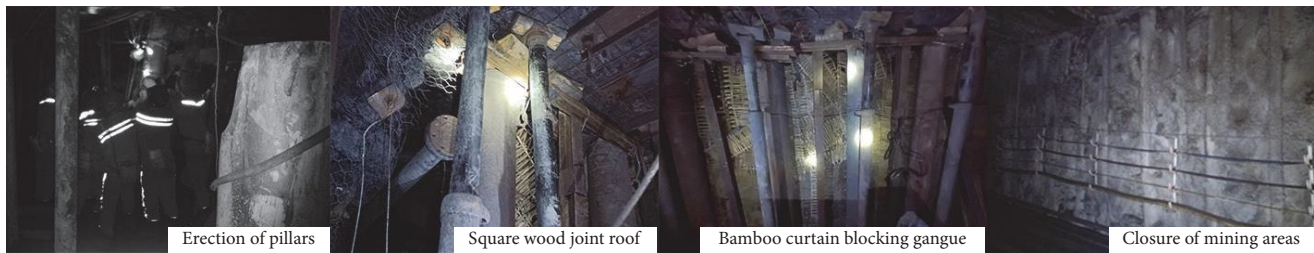
FIGURE 18: Roadway side support.
