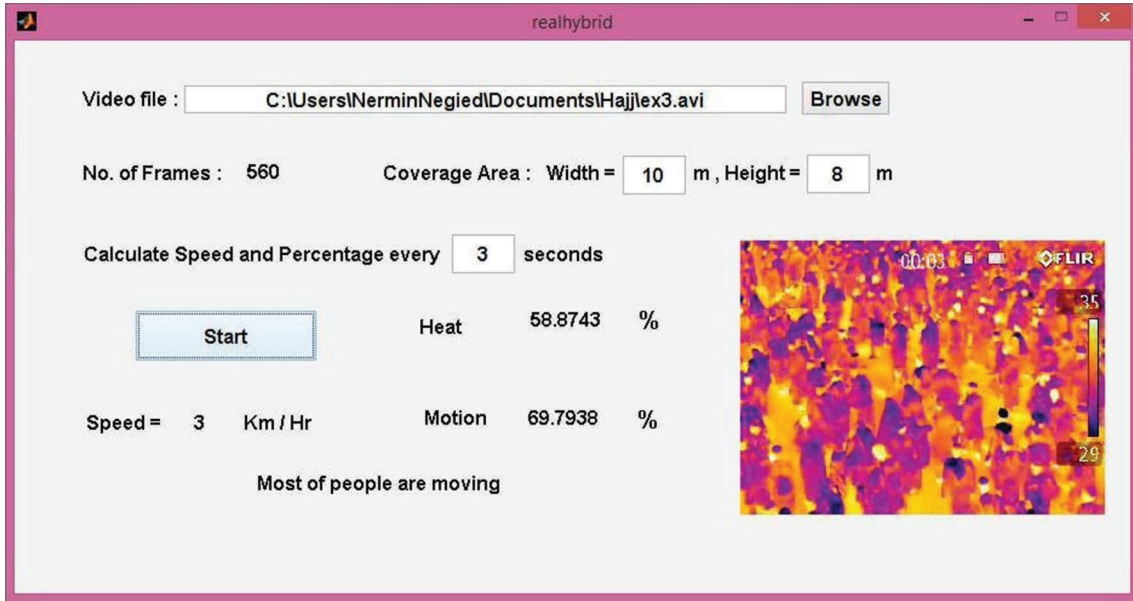
FIGURE 20: Density calculation using a thermal image utilizing heat signature and background subtraction by HSBS [14].
