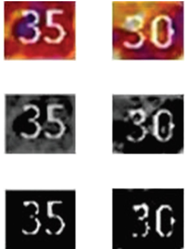
FIGURE 8: Sample of cropped boxes represent upper and lower temperature degrees, converted from RGB to gray and then to binary levels.
