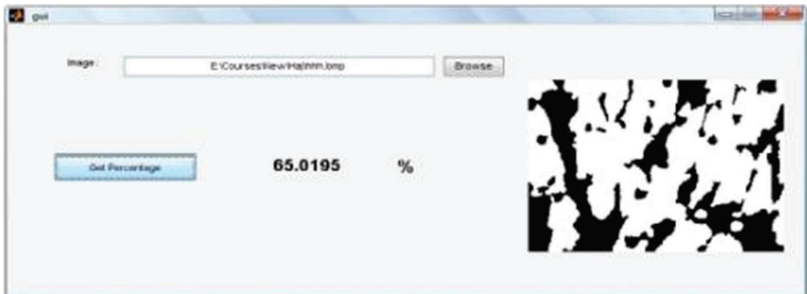
FIGURE 19: Density calculation using a thermal image utilizing background subtraction by Abu Arafah [20].
