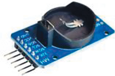
FIGURE 5: RTC DS3231 RTC (as adopted from https://learn.adafruit.com/adafruit-ds3231-precision-rtc-breakout ).
