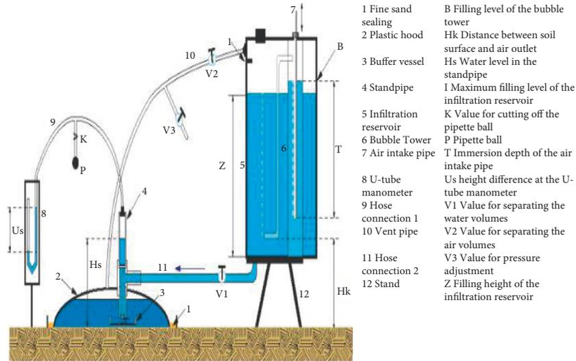
FIGURE 3: Hood infiltrometer [31].
