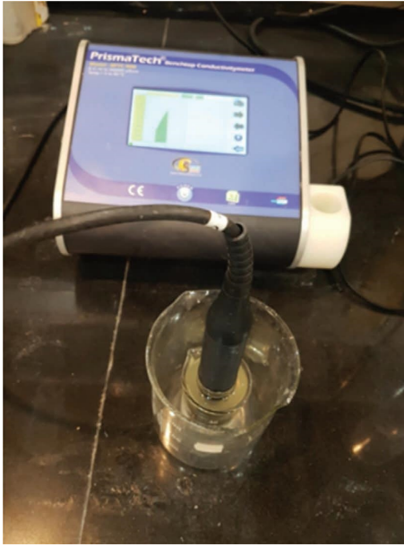
FIGURE 4: Measuring urease activity for UCE using an electrical conductivity meter.
