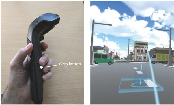
FIGURE 4: Interacting with the HTC Vive controller for the teleportation technique (*left*) and a view of the virtual environment (*right*). Video demonstration of virtual navigation: <http://boletsis.net/vrloco/teleport/>.
