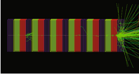
FIGURE 4: Geant4 simulation for a 50 TeV tau penetrating interleaved detectors made by 3 layer RPC (in blue), lead tungstate (PbWO 4 , in green), and copper (in red), each with 20 cm's length. The energetic tau flies like a muon and then decays into 3 charged pions and neutrinos. The gamma rays shows in green, electrons in red, and electron neutrinos in white.
