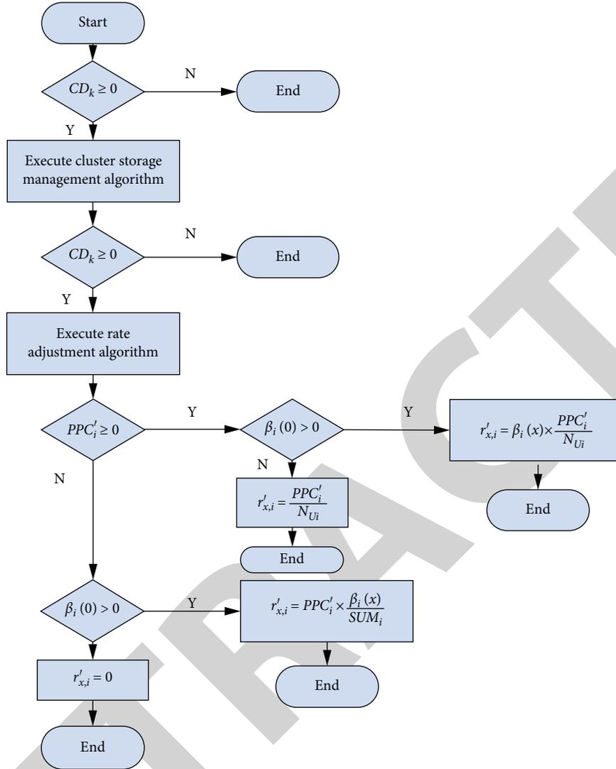
FIGURE 2: Process flow chart of the OFMNSE algorithm.
