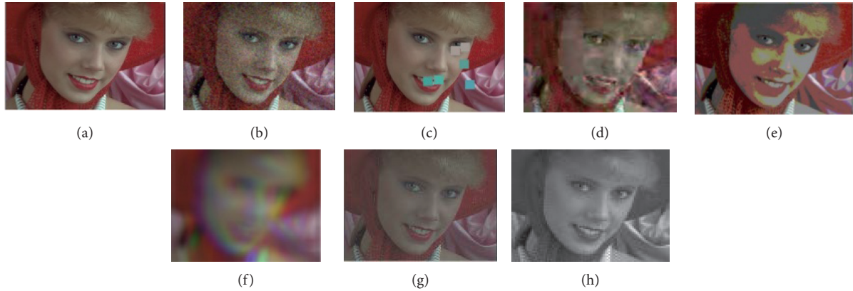
FIGURE 3: Examples of different types of distortions. (a) Reference image. (b) Spatially correlated noise. (c) Local block-wise distortions. (d) Comfort noise. (e) Quantization noise. (f) Chromatic aberrations. (g) Contrast change. (h) Change of color saturation.
