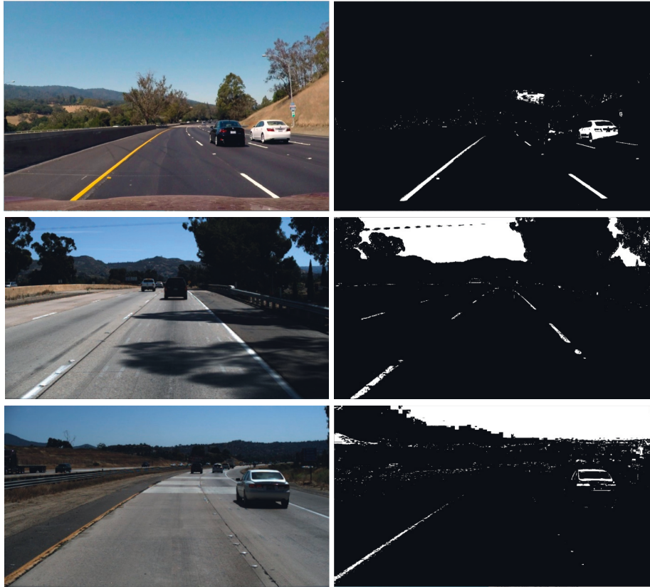
FIGURE 5: An example of the HLS threshold.
