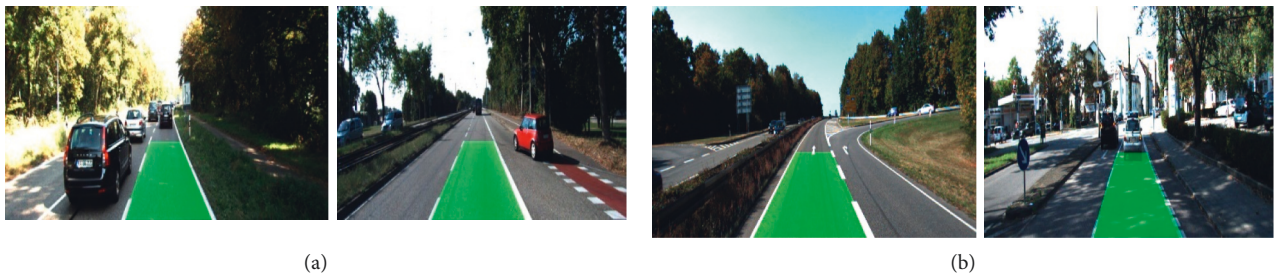
FIGURE 19: Results of lane detection for different conditions: (a) shade and (b) good lighting in the KITTI dataset.
