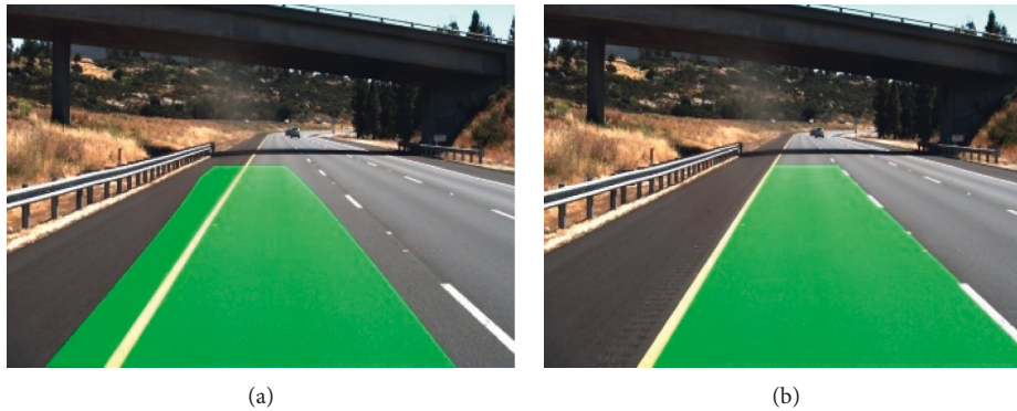
FIGURE 21: Result of lane detection with window sizes of (a) 50 pixels and (b) 100 pixels in the TuSimple dataset.
