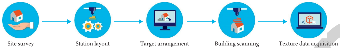
FIGURE 4: Flow chart of 3D scanning data acquisition.
