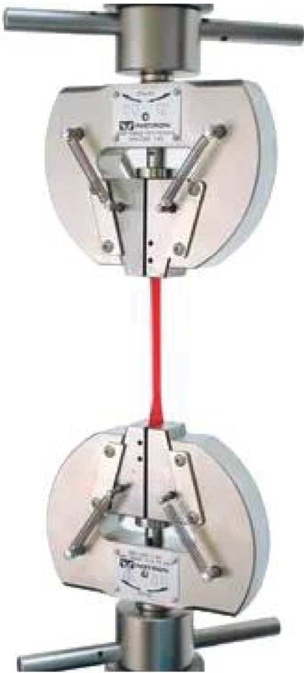
FIGURE 3: Bonding force tensile test.
