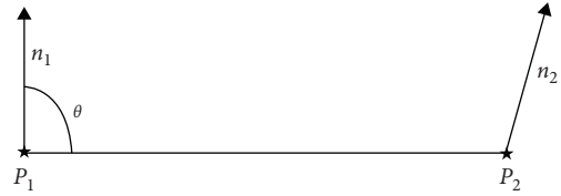
FIGURE 3: The included angle between the line segment and the normal vector of the endpoint.
