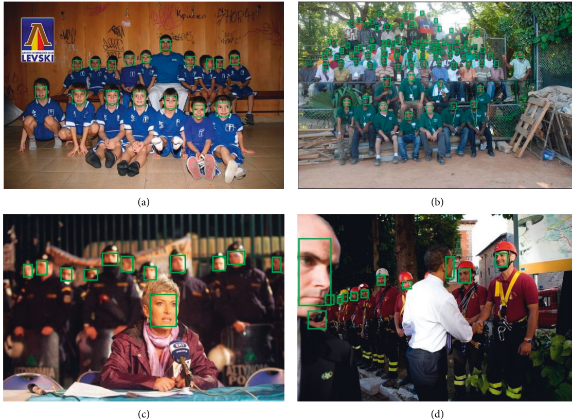
FIGURE 7: Detection results on the WIDERFACE set. (a) Light change. (b) Dense small faces. (c) Fuzzy scene. (d) Blocking faces.
