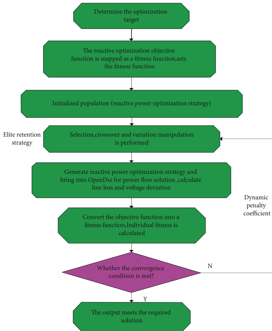
FIGURE 7: The reactive power optimization process of the distribution network is based on improved GA.
