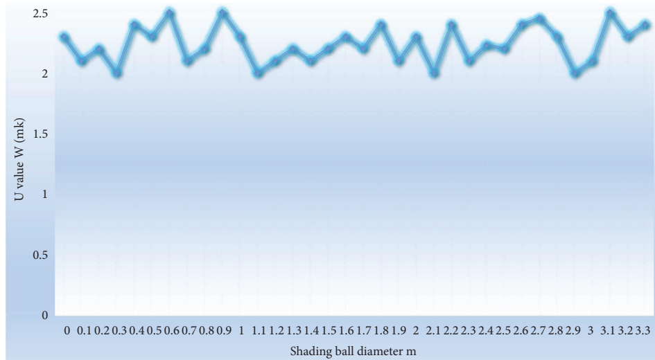
FIGURE 3: Simulation U value of dynamic skin driven by PCM of various sizes in summer shading state.
