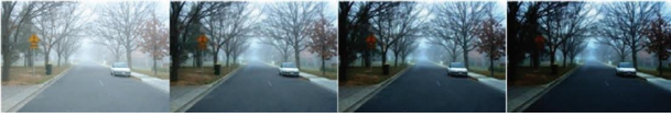
FIGURE 3: Image overexposure processing. The \gamma values from left to right are 2, 3, and 4.
