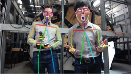
FIGURE 2: OpenPose human keypoints detection [39].
