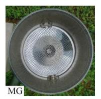
Figure: Comparison of screen strainer and mesh size between RG3-M and manual gauge. Note that the screen mesh of RG3-M usually forms a thin liquid film during rainfall which easily makes raindrops rebounding out of the strainer. Thus, more raindrops splash out of the RG3-M gauge than those of manual gauge, especially for the storm with high intensity.
