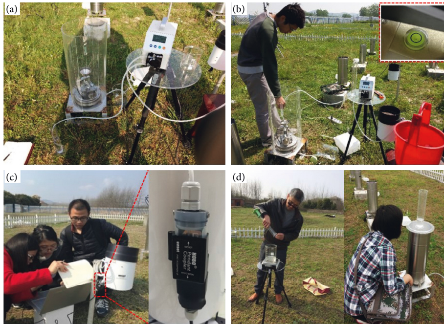
FIGURE 2: (a) Peristaltic pump used for calibration. (b) The calibration of tipping bucket rain gauge. (c) Obtaining the data from RG3-M (left), the data logger (right). (d) Comparison of precipitation measurement for the manual gauge: weighting method (left) and horizontal visual method (right).
