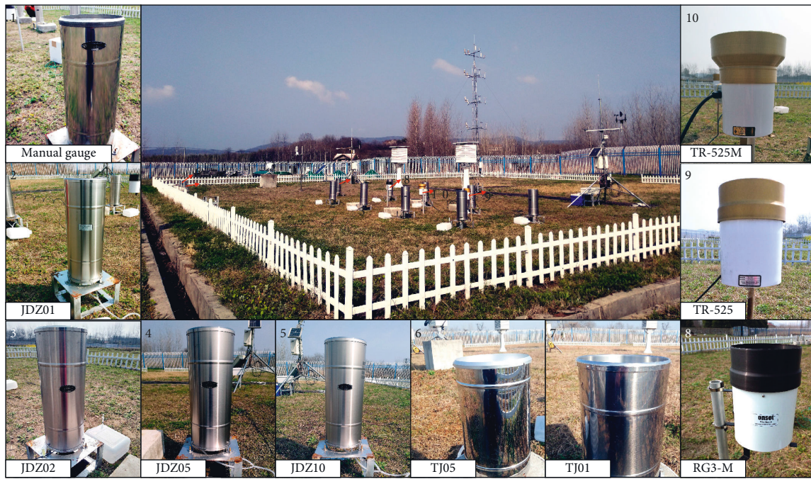
FIGURE 1: (a) Field view of the Chuzhou hydrological experiment station, (b) distribution of 10 models rain gauges, and (c) the site of hydrometeorological observation field.
