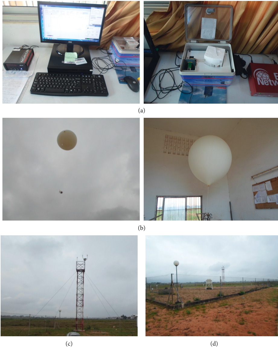
FIGURE 2: Material for measuring wind parameters. (a) Radiosonde data station and ground check. (b) The release of the probe and the balloon. (c) Cup anemometer and weather vane located on a mast of 10 m. (d) Experimentation site over the coast of Cotonou, Benin.
