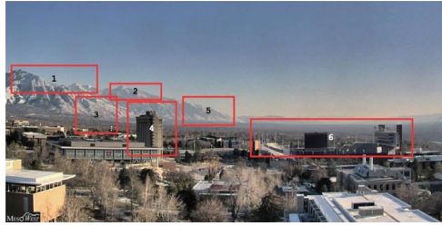
FIGURE 14: Salt Lake City (University of Utah) webcam image facing south, showing marked segments used for evaluation (refer to Table 2). Frames 1 and 2: top of the mountains for “hills obscured” determination. Frame 3: suburbs and mountain ridge base, including Jacks Peak and Pencil Point, situated 5 km away. Frame 4: social and behavioral sciences building, located 500 meters away. Frame 5: daylight visibility assessment. Frame 6: Rice-Eccles Stadium, situated 650 meters away.
