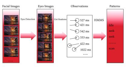
FIGURE 3: Flow chart of image feature extraction.
