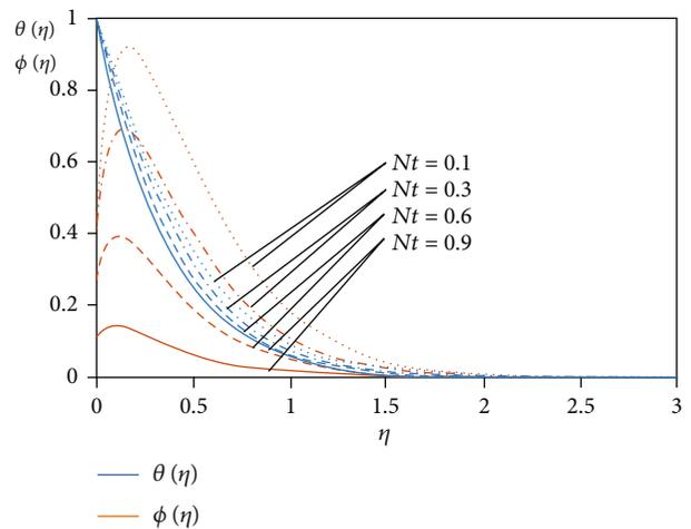
FIGURE 8: Concentration and temperature profiles affected by thermophoresis parameters.
