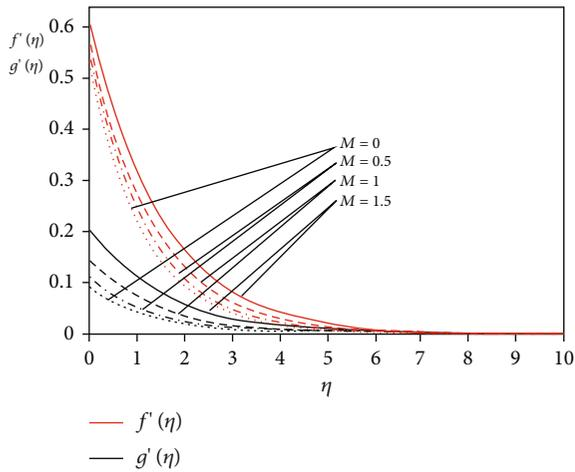
FIGURE 3: Velocity profiles affected by magnetic field parameters.
