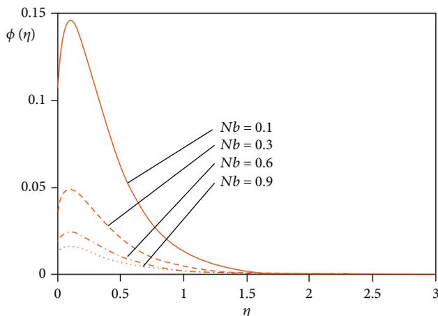
FIGURE 9: Concentration profiles affected by Brownian motion parameters.
