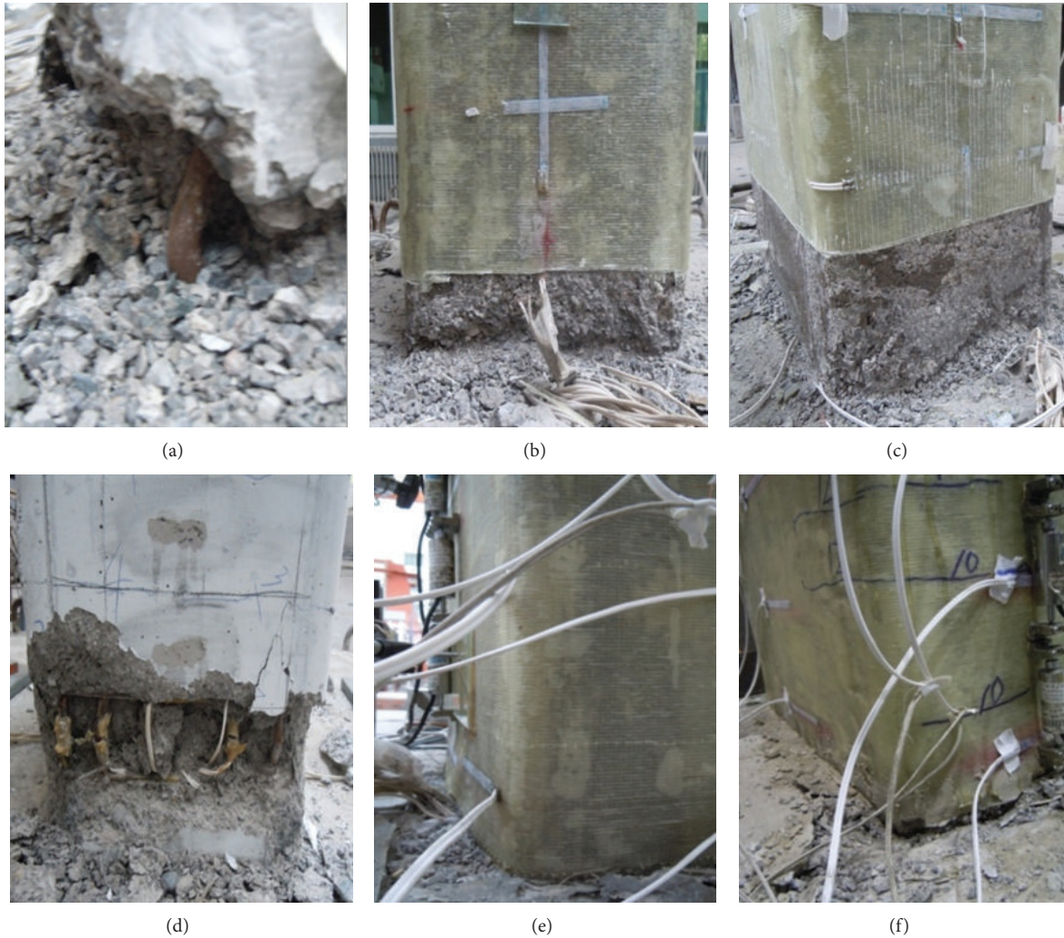
FIGURE 2: Failure modes of specimens (a) SU-1, (b) SHG-2, (c) SHG-3, (d) LU-1, (e) LHG-2, and (f) LHG-3.
