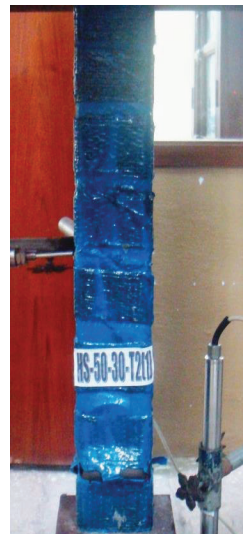
FIGURE 9: Failure mode of column HS-50-30-T2(1).
