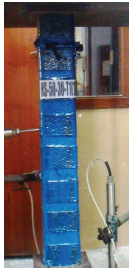
FIGURE 8: Failure mode of column HS-50-30-T1(1).
