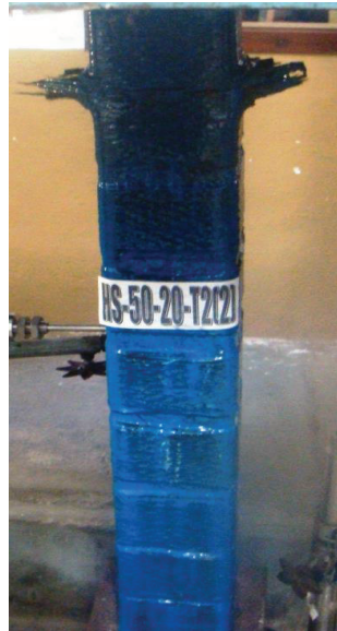
FIGURE 6: Failure mode of column HS-50-20-T2(2).
