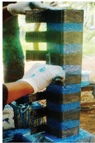
FIGURE 2: Squeezing of resin by steel roller.
