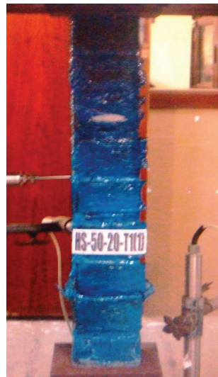
FIGURE 5: Failure mode of column HS-50-20-T1(1).
