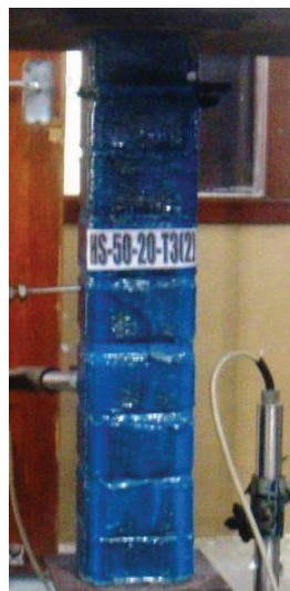
FIGURE 7: Failure mode of column HS-50-20-T3(2).
