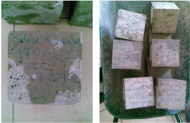
FIGURE 3: Generation of cavities on surfaces of the plain concrete specimen due to sulfate reactions.
