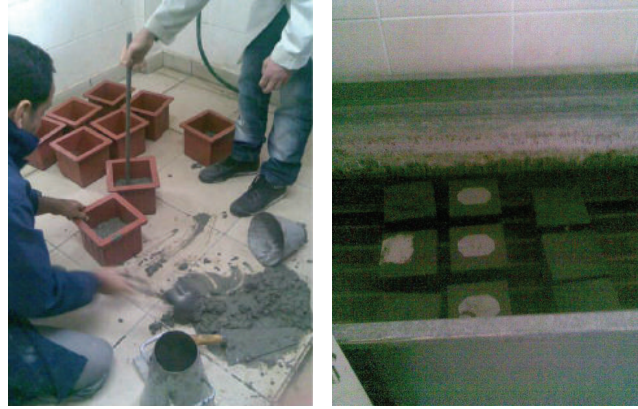
FIGURE 2: The mixing of fresh concrete and curing processes.
