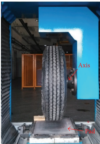
FIGURE 4: Static loading test.
