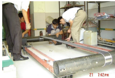
(f) Check-up on the fixation before the jack-up process
