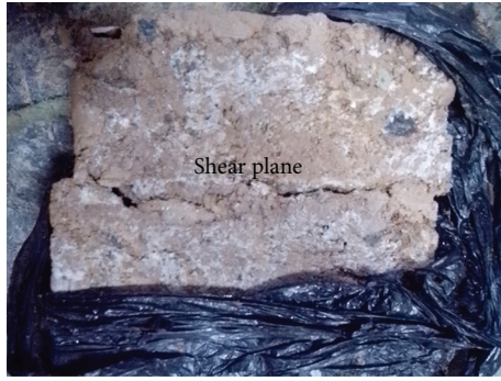
FIGURE 3: Representative shear plane of tested specimen.
