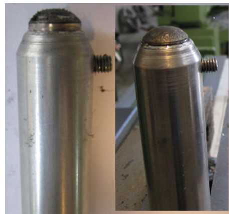
FIGURE 3: Spark machined magnet with its fixture.
