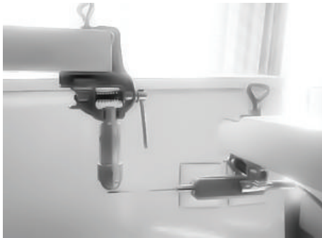
FIGURE 7: Measuring magnetic flux density at 2 mm from the surface of iron hemisphere.
