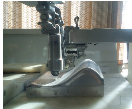
FIGURE 11: Measuring magnetic flux density between magnet and workpiece surface.
