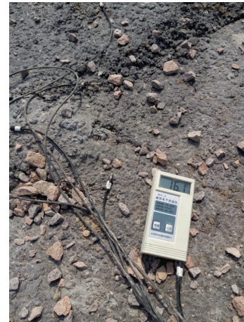
FIGURE 8: Temperature rise procedure test system.
