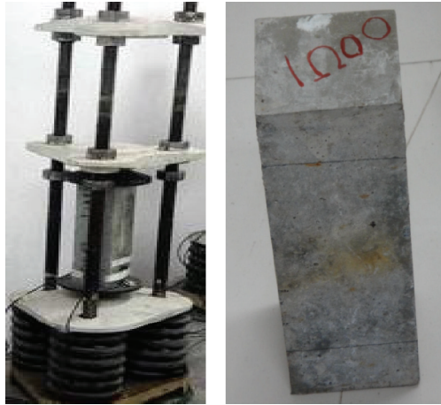
FIGURE 7: Creep loading test and standard concrete sample.
