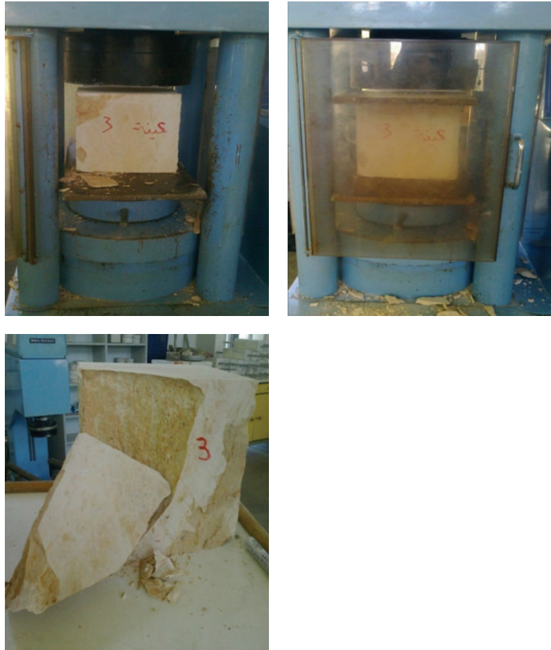
FIGURE 5: Stone sample 3 under compressive strength testing.
