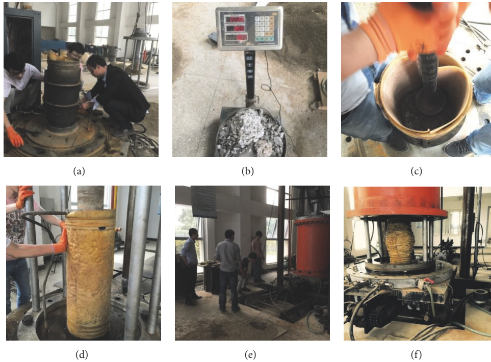
FIGURE 4: Triaxial compression test procedure: (a) mould tube installation, (b) sample weighing, (c) sample layer vibrating chamber, (d) sample vacuum forming, (e) sample saturation, and (f) sample shear failure.
