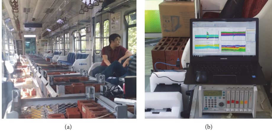
FIGURE 10: Test vehicle and data acquisition system for track test.
