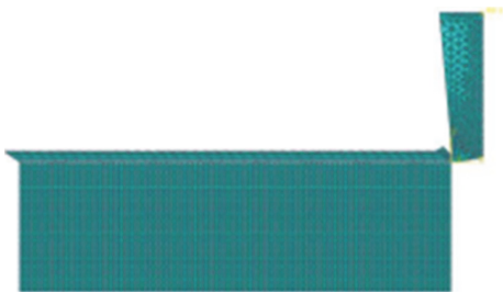
FIGURE 4: Finite element model of wheel tread reprofiling.
