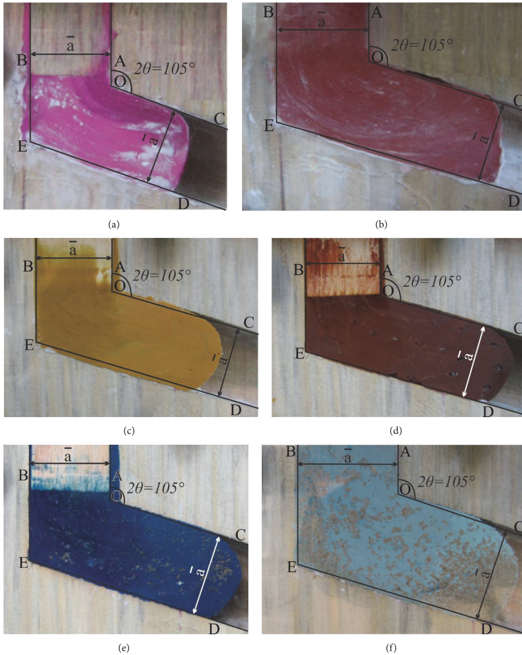
FIGURE 1: The flow of physical plasticine models of polymer materials through an ECAE die AOC-BED of Segal geometry with channel intersection angle \angle(BED) = \angle(AOC) = 2\theta = 105^\circ : (a), (b), (c) the flow of uniform plasticine workpieces; (d) the flow of plasticine workpiece with additional solid markers at the front surface of workpiece in the shape of the hard spots; (e), (f) the flow of plasticine workpieces with additional dispersed particles on the front surfaces of workpieces in the form of partially immersed fine sawdust.
