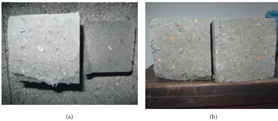
FIGURE 5: Section of steel fiber-reinforced silica fume concrete.
