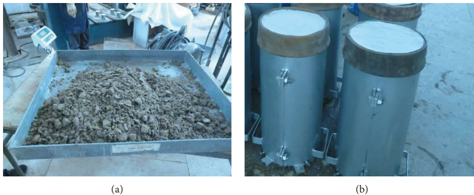
FIGURE 2: (a) Mixed materials; (b) samples of CSG material.
