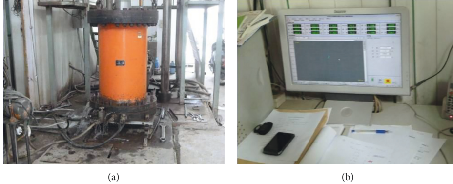
FIGURE 1: TYD-1500 triaxial tester, which should be listed as (a) large-scale dynamic triaxial tester; (b) data acquisition system.
