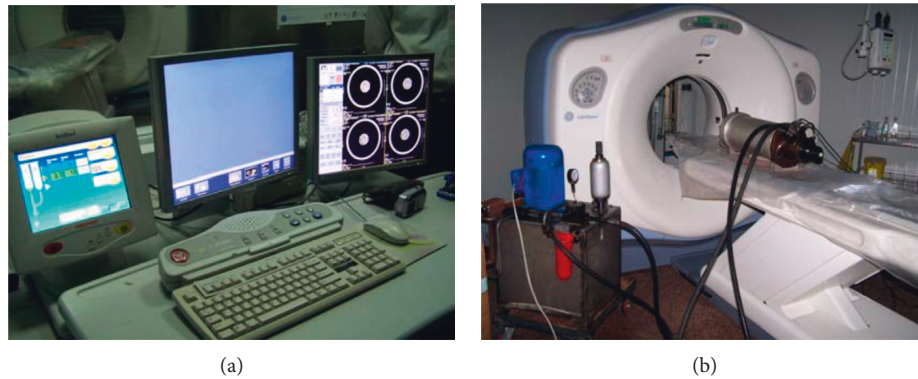
FIGURE 2: The CT machine and loading instrument. (a) CT output display. (b) CT machine and power loading instrument.
