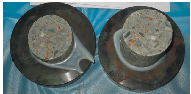
FIGURE 18: The failure of the specimen under dynamic tension loading.
