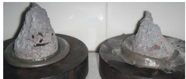
FIGURE 14: The failure of two specimens subjected to dynamic pressure loading.
