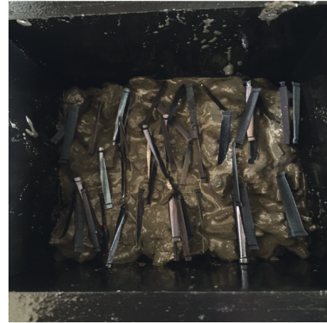
FIGURE 1: Directionally distributed steel fibres in a concrete specimen.
