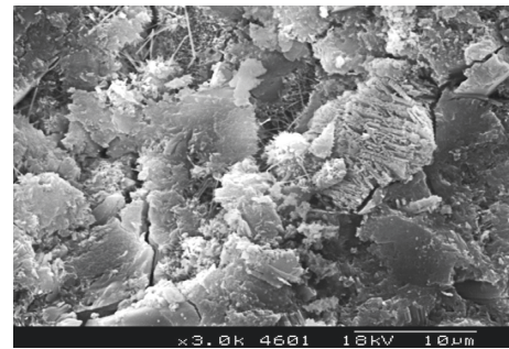
FIGURE 10: Microstructure of GC3 (proper amount of SF, at 28 days).
