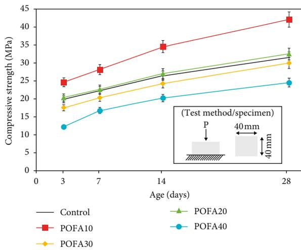
FIGURE 4: Compressive strength of mortars containing mPOFA.
